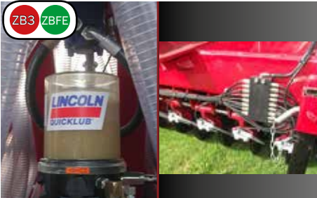
Automatic lubrication system for low maintenance.
