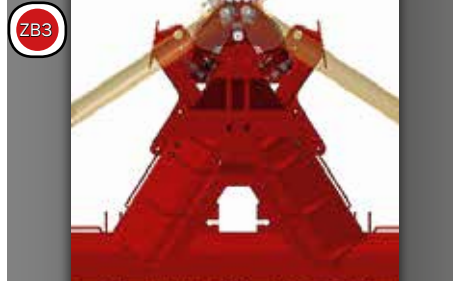
The centre pivot, to stay in contact with the soil even with undulations.
