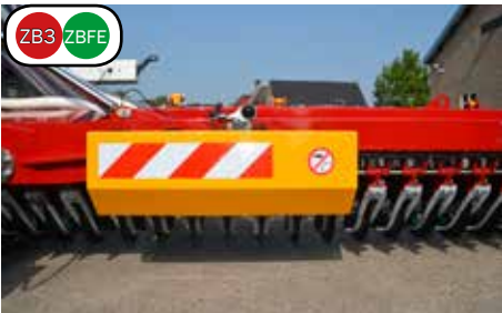
Reflective automatic retractable disk protection shields.
