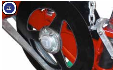
Greasable bearings for a long lifespan
