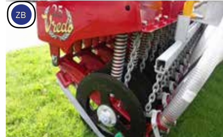
Mechanical pressure on the soil for optimal adaptation.
