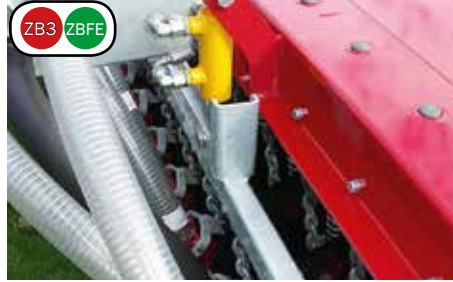
Hydraulic shut-off valves for a clean operation
